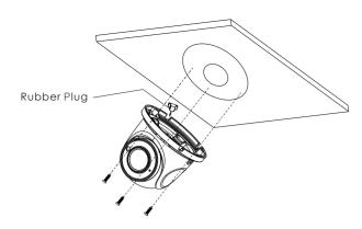
③ Adjust the camera to obtain an optimum angle by loosening the fixed screws. Before adjustment, preview the image of the camera on a monitor. After that, tighten the fixed screws.
