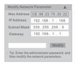
For example, the IP address of your computer is 192.168.1.4. So the IP address of the camera shall be changed to 192.168.1.X and the gateway shall be changed to 192.168.1.1. After modification, please enter the password of the administrator and click "Modify" button to modify the settings.
