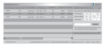
③ Modify the IP address. The default IP address of this camera is 192.168.1.168. Click the information of the camera listed in the above table to show the network information on the right hand. Modify the IP address and gateway of the camera and make sure its network address is in the same local network segment as that of the computer. Please modify the IP address of your device according to the practical situation.
