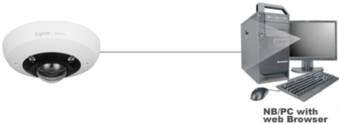
Figure 6 Camera Network Topology Type I.
