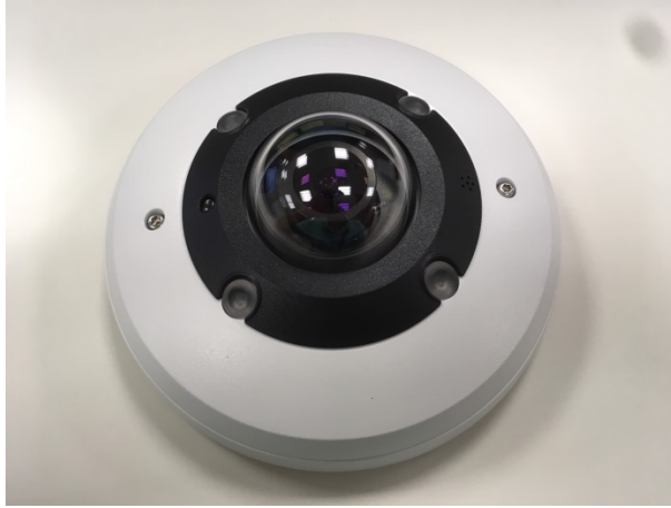
Figure 13 : Top cover securely fitted
