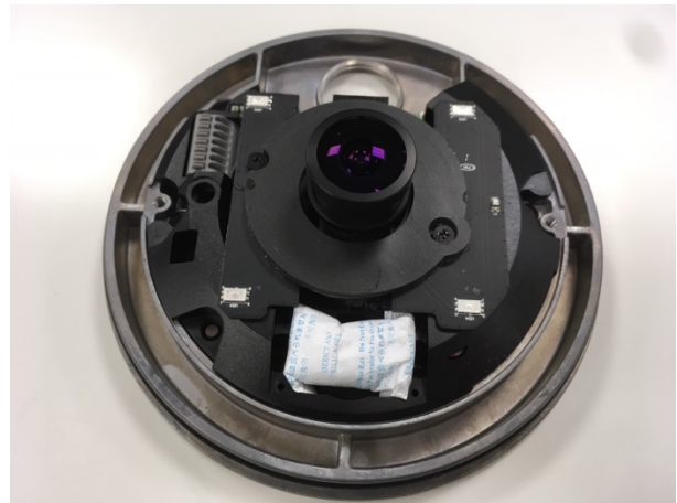
Figure 12 : Desiccant bag placement location (left side) Desiccant bag in the camera (right side)
