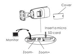
⑥ Install the cover back to the camera and fix it firmly with the screws. (Note that the cover should not be installed unevenly.)
