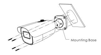
④ Bracket adjustment. Before adjustment, preview the image of the camera on a monitor (See the left figure of step ⑤) and then loosen the fixed screws to adjust the view angle of the camera. After that, tighten the fixed screws.
