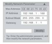
For example, the IP address of your computer is 192.168.1.4. So the IP address of the camera shall be changed to 192.168.1.X and the gateway shall be changed to 192.168.1.1. After modification, please enter the password of the administrator and click "Modify" button to modify the settings.
